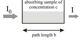
Absorption instruments can usually display the data as either transmittance, %-transmittance, or absorbance.
